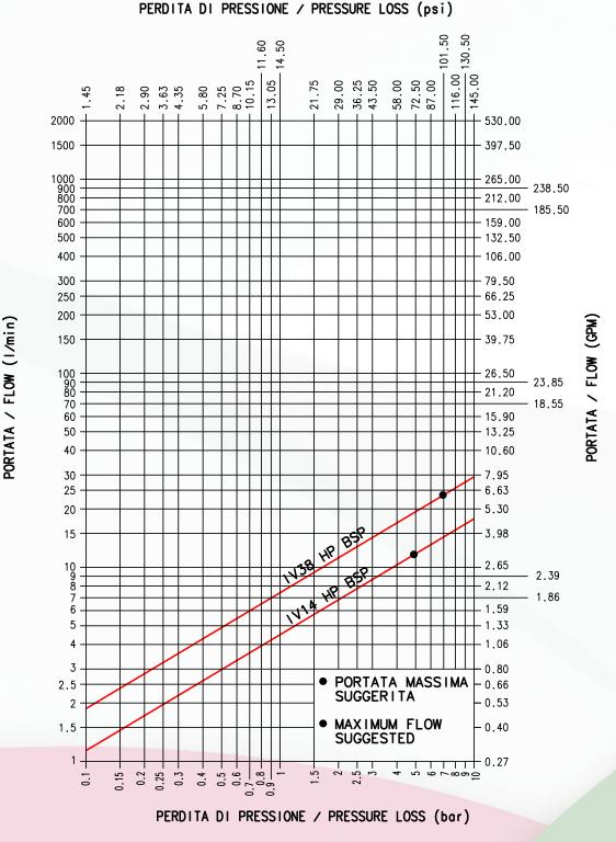
FLUIDO: OLIO ISO VG32 TEMPERATURA: 40°C VISCOSITA': 28.8-35.2 mm<sup>2</sup>/s FLUID: OIL ISO VG32 TEMPERATURE: 40°C VISCOSITY: 28.8-35.2 mm<sup>2</sup>/s
